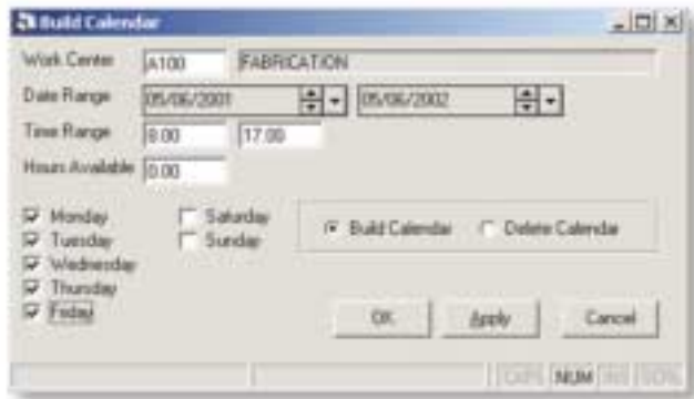
Build Calendar creates a calendar for a work center showing when the work center is available for work.
