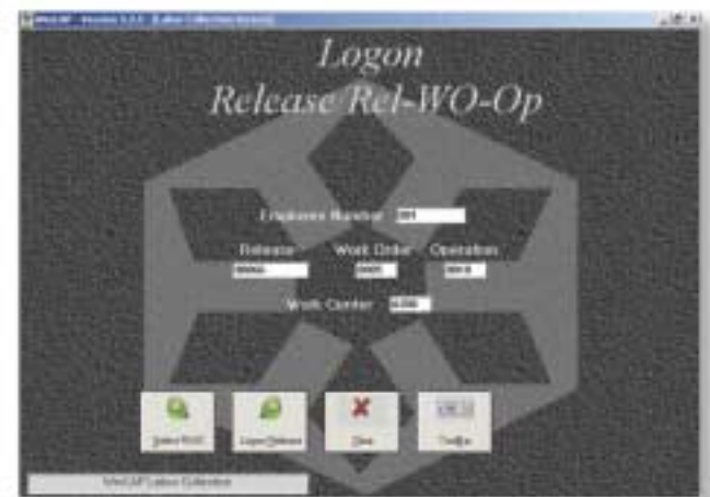
WinCAP's logon screen allows the user to logon to a release or release-work order-operation through manual or bar-coded data entry.
